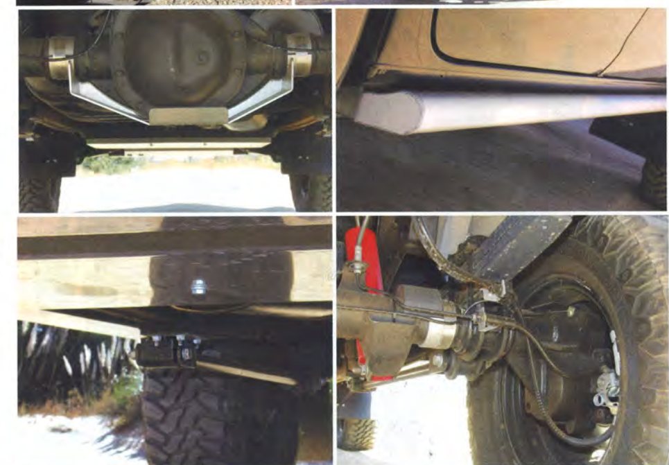
The notable upgrades to the Amarok Xtreme include 17-inch steel rims, heavy-duty underbody protection plates, rock sliders and the portal axle set-up. Note the close-up of the hub reduction in the picture, bottom right.
